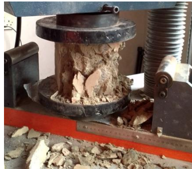
Figure 4 Compression testing of concrete specimens
